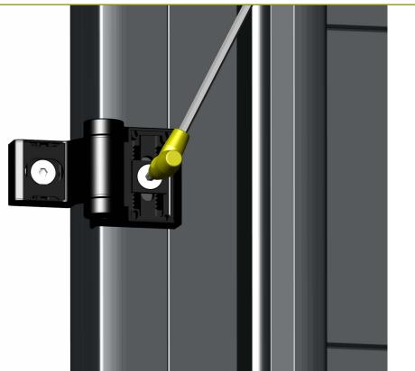
Check that the bolts on both sides of the hinges are placed in the middle of the hinges and make sure that the bolts are slightly tightened.
